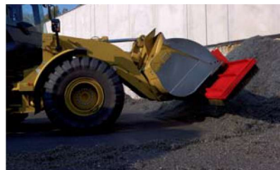
Industrial Brush Mod. 4 mt Attack for Bulldozer: 4000 mm Width 1000 mm Length 750 mm Depth 1200 kgs Weight
